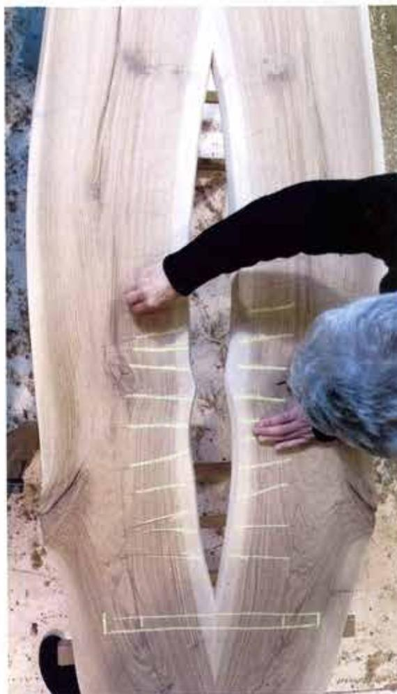
MARKED BOARDS. The patriarch uses a piece of chalk to mark the process to be applied and where to cut.
